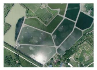
Aerated lagoons (AL) in Chiang Mai. This treatment method is typical for this region. ALs are easy and inexpensive to construct and operate. With this method, waste is degraded by various microbiological populations and pathogens can be effectively removed by aeration or exposure to sunlight. ©GIZ
