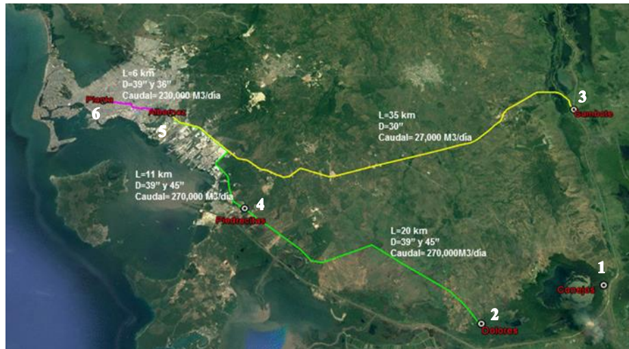
Image 1. Aguas de Cartagena Drinking Water System. Where 1 is the Conejos pumping station, 2 is the Dolores pumping station (flow=270.000 m 3 /day), 3 is the Gambote pumping station (flow=27.000 m 3 /day), 4 is the Piedrecitas pumping station (flow= flow=270.000 m 3 /day), 5 is the Albornoz station (flow= flow=230.000 m 3 /day) and 6 is the water treatment plant.
