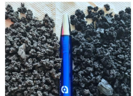
Figure 6: Biochar from pyrolysis and Biosolids 90% Dry Matter - Photo by Ivan Volund
